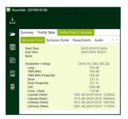
Multiple measurement runs can be downloaded and stored. For any elected run, a summary screen provides essential information such as date and measurement run time along with the measurement protocol e.g. to ISO, multiple US or customer requirements. It also shows the measured and projected 8 hour dose results plus many other parameters for comparison with the regulatory action levels.
